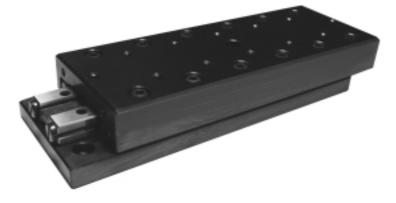
PM frictionless precision slides type RTN and RTL are pre-loaded linear motion components, ready for mounting. The well proven design of this model offers a wide range of benefits as for example; high rigidity, no stick-slib effect and an unprecedented precision in linear movement thanks to the installation of a double-sided track-rail on the slide-base which eliminates machining errors on the slide-base.
