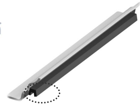
[Bottom retainer - Unified seal]
