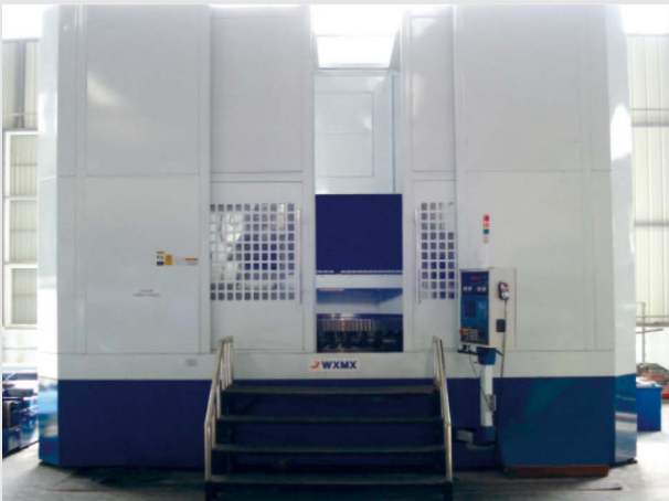
MX-1800 立式数控磨床加工中心 MX-1800 Vertical CNC grinding machine processing center
