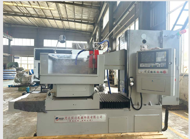
MSK7363 数控卧轴圆台平面磨床 MSK7363 CNC surface grinding machines with horizontal wheel spindle and rotary table
